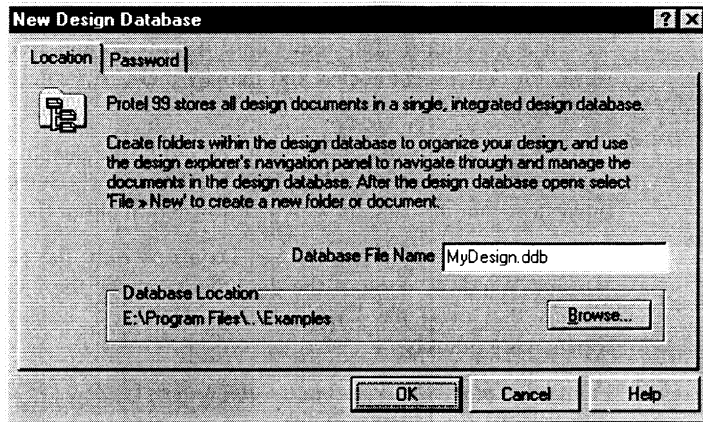
Creating a New Design Database, enter the name and change the location if necessary
